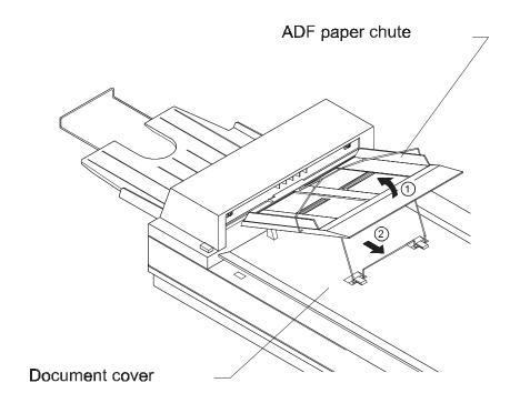
Figure 2-4 Setting the ADF Paper Chute
